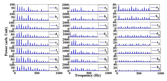
FIG. 4. FFT power spectra of the signals of the floating potential fluctuations in regimes I, II, and III at 250 V.
