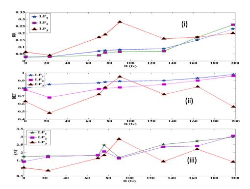
FIG. 7. Recurrence measures (i) RR, (ii) DET, and (iii) ENT of the floating potential fluctuations with respect to different magnetic fields.
