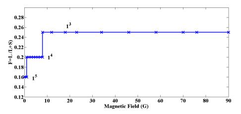
FIG. 11. Devil's staircase represents the changes in the firing number with the magnetic field at 240 V.
