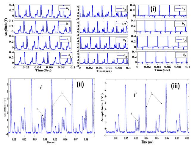
FIG. 2. (i) Signal of the floating potential fluctuations obtained by the inner  $(a_1)$ – $(d_1)$ , the middle  $(a_2)$ – $(d_2)$ , and the outer Langmuir probes  $(a_3)$ – $(d_3)$  in various magnetic fields: (a) 0 G, (b) 4 G, (c) 8 G, and (d) 12 G at 240 V. (ii) and (iii) Shows the expanded view of the signals  $a_2$  and  $d_2$  of (i).
