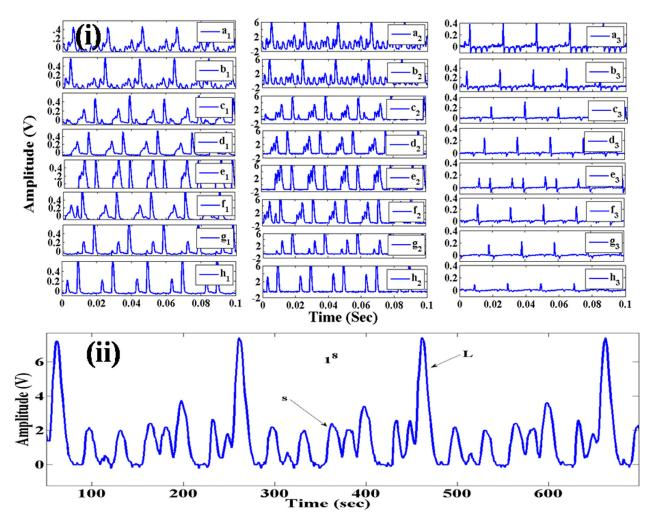
FIG. 3. (i) Represents the time series of the floating potential fluctuations obtained by the inside  $(a_1)$ – $(h_1)$ , the middle  $(a_2)$ – $(h_2)$ , and the outside Langmuir probes  $(a_3)$ – $(h_3)$  in various magnetic fields: (a) 0 G, (b) 23 G, (c) 70 G, (d) 76 G, (e) 90 G, (f) 132 G, (g) 164 G, and (h) 198 G. (ii) Representation (Zoom) of the signal  $a_2$  at 250 V.
