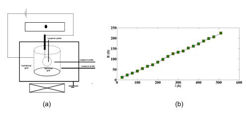
FIG. 1. (a) Schematic diagram of the experimental setup. (b) Calibration curve for the current passes through the Helmholtz coil versus the produced magnetic field.
