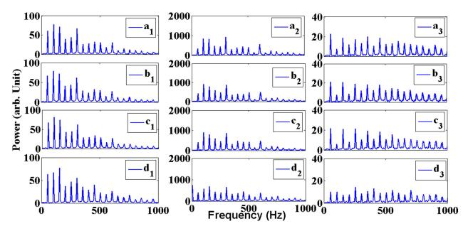
FIG. 5. FFT power spectra of the signals of the floating potential fluctuations in regimes I, II, and III at 240 V.
