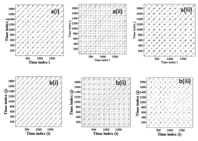
FIG. 6. (a) and (b) Recurrence plot of the floating potential fluctuations obtained in (i) regime I, (ii) regime II, and (iii) regime III at (a)  $250 \,\mathrm{V}$  and (b)  $240 \,\mathrm{V}$  with B=0.
